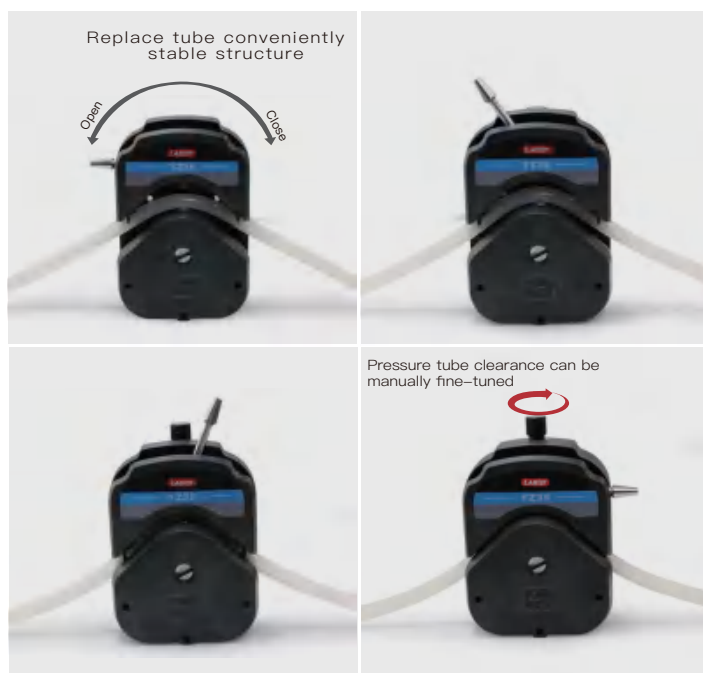
Installation tube method
